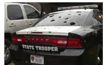
Hail Damage to Back Glass
